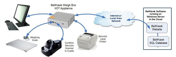
The BellHawk Weigh Box (WeighBox) IIOT appliance enables weighing scale data to be captured automatically and used as part of BellHawk Online data entry transactions.
