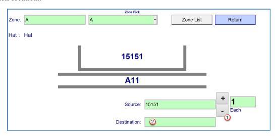
From this screen, the user scans the Source bin/shelf location and then the barcode on the destination container, such as basket, box, or pallet to confirm the transfer. The system confirms that the Source contains the correct parts and that the Destination contains only parts for the Pick Order selected at the beginning of the zone picking process. Otherwise the user is given an error message on their mobile display and has to repeat the picking process for the part.
