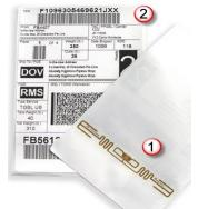
When an RFID tag is detected by the RFID tag reader on a specific antenna, the tag number and antenna is reported from the RFID tag reader to the RFID box. The RFID box then translates from the RFID tag number to the specific container in BellHawk and translates from the antenna location stored in BellHawk to the new physical location of the container, which the RFID box then records into the BellHawk database through the BellHawk website's web services interface.
