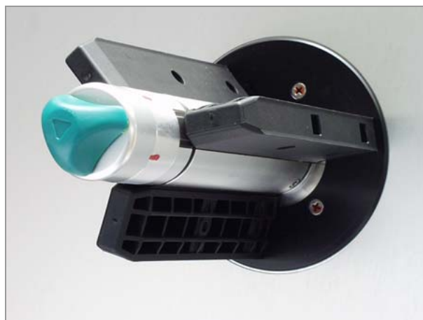
[72] Position of core adapter for 101.6 mm core diameter.
