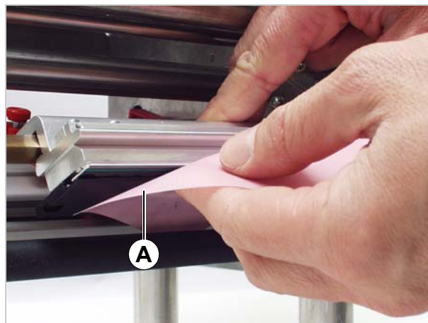
[96] Clean the printhead with the cleaning strip.
