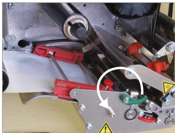
[57] Shut the lever for the pressure roller.
